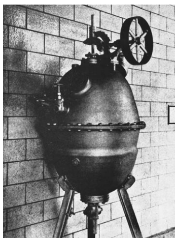
Figure 4. The autoclave that served to produce Bakelite in Yonkers (1907–1909).
